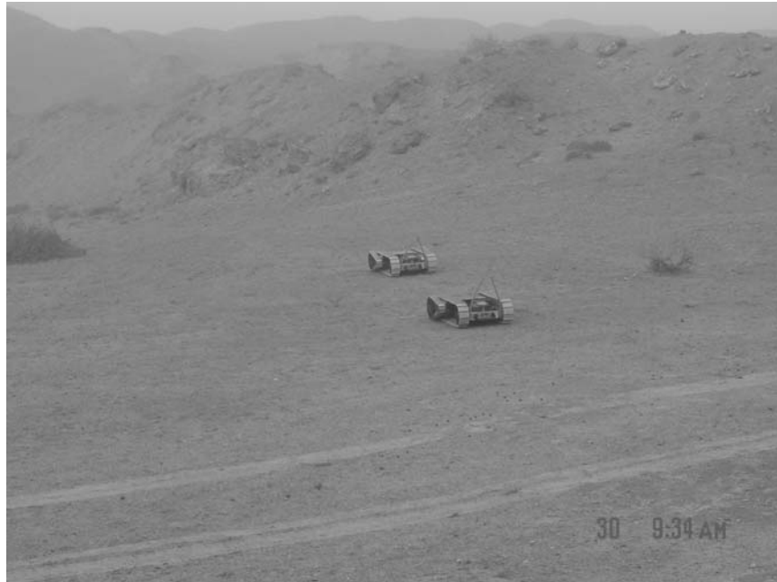
Figure 1: PackBots with CHARS Payloads Searching for Chemical Weapons in Iraq
