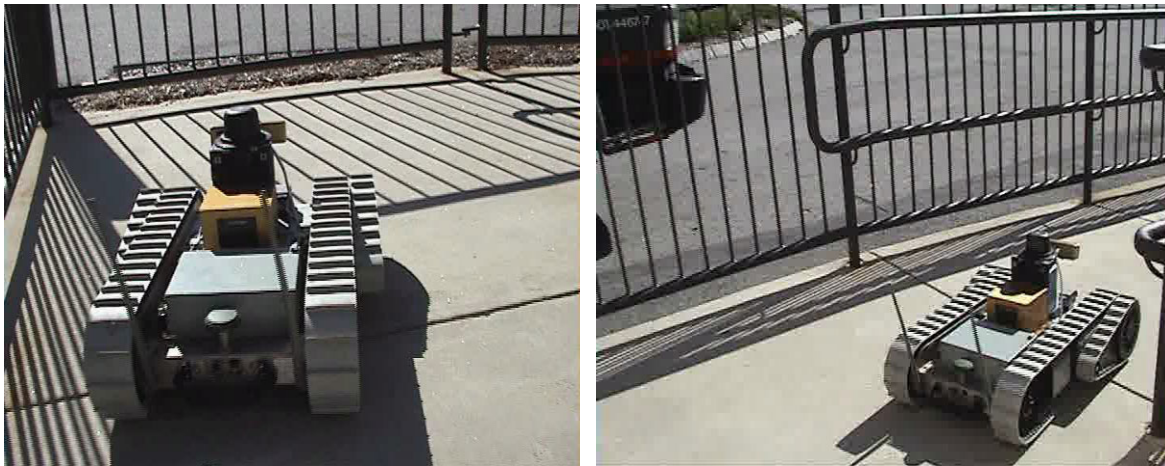
Figure 4: PackBot Wayfarer steers down 180-degree handicap ramp
