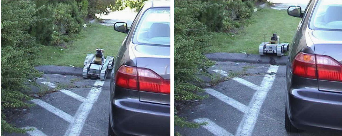
Figure 5: PackBot Wayfarer steers through narrow gap between bushes and car
